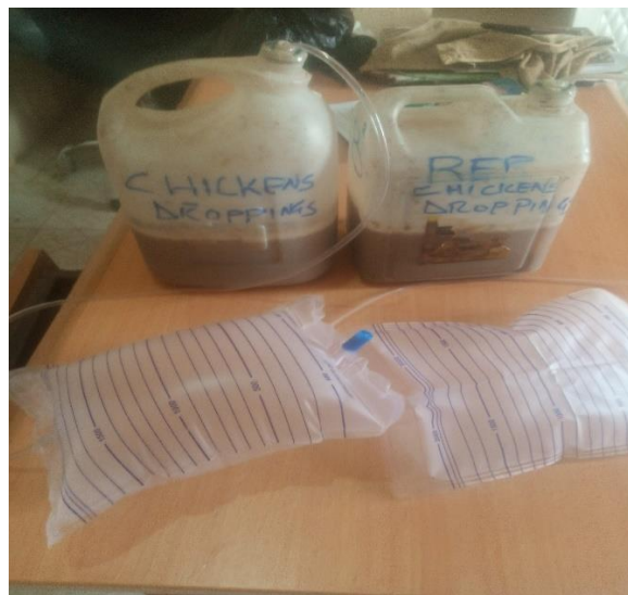
Plate 2: Biogas in a urine bag collector
