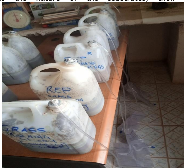
Plate 1: Biogas production in progress
