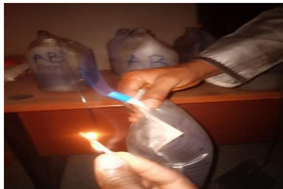
Plate 4: Blue Flame at Methanogenesis stage
