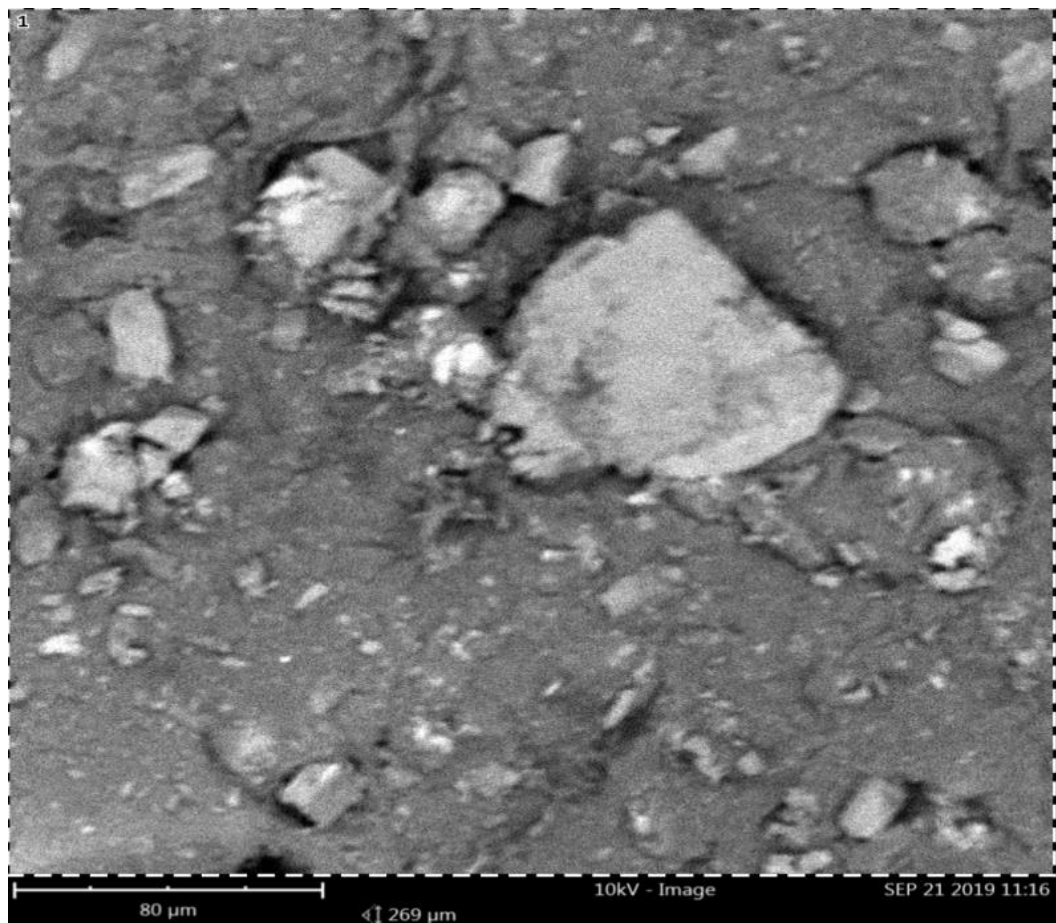
Plate 1: SEM Analysis of Nanoparticles Immobilized Watermelon Rinds
