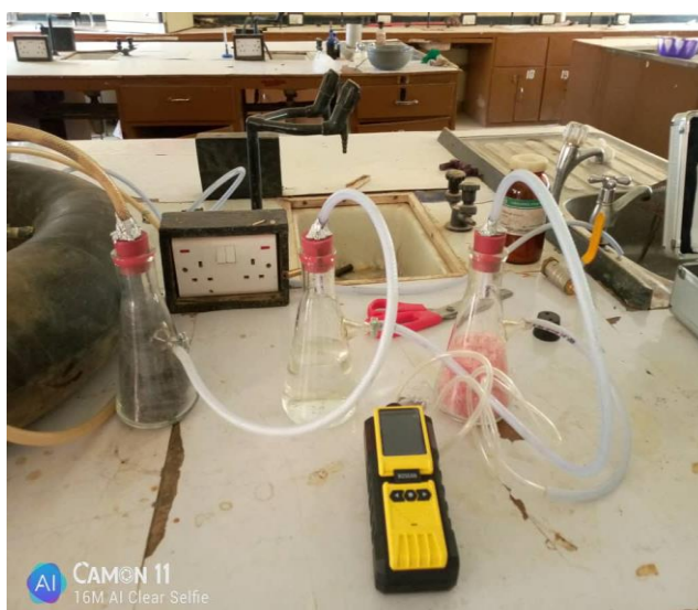
Plate II: Laboratory scale purification and upgrading of biogas to bio-methane
