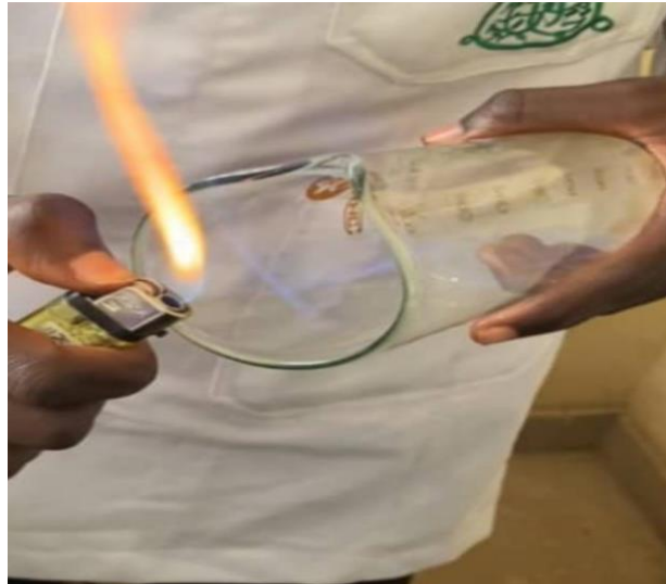
Plate II: Flammability (Quality) Test for Methane Content of the Control Set-up (without supplementation)
